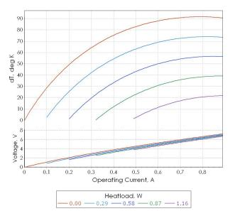
**Note**: Performance data is specified at optimal optimal conditions (TEC hot side is stabilized at ambient temperature). Any heatsink thermal resistance is not included into estimations. Use TECCad Software for estimations under different conditions.
